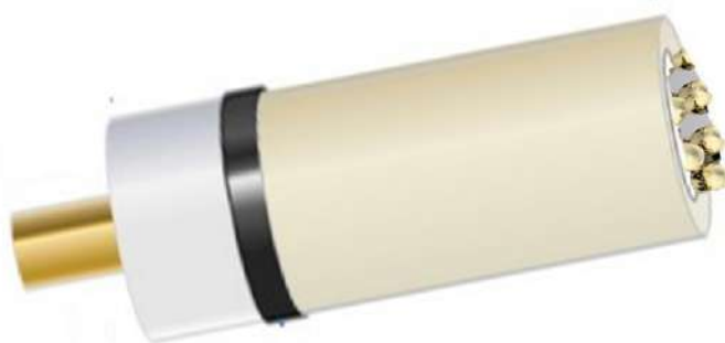
Figure 2. Schematic representation of a working electrode, with active electrode surface modified with gold nanoparticles
